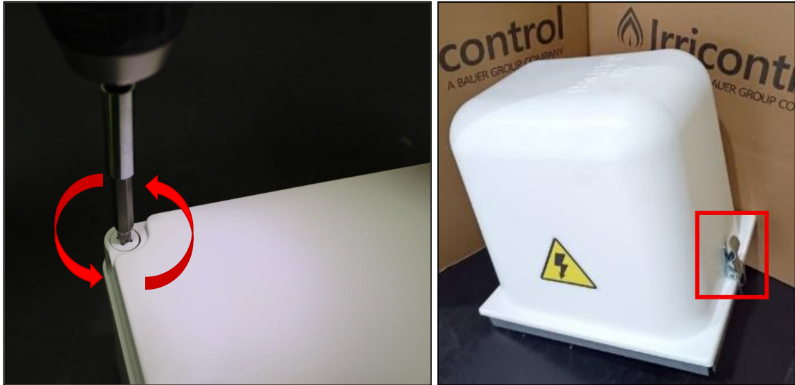
Figure 16 - Opening of the plastic boxes and removal of the control cabinet cover.
