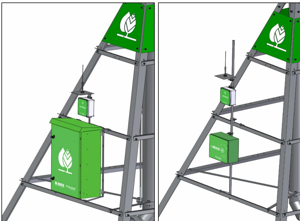
Figure 1 - 4G Module G2 Installation on the center tower - SmartConnect G2 and Nexus G2.
