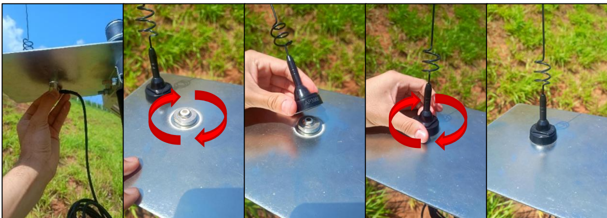
Figure 14 - Antenna Installation on the support.
