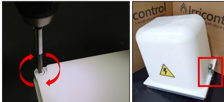
Figure 27 - Closing the GPS plastic box and the control box.
