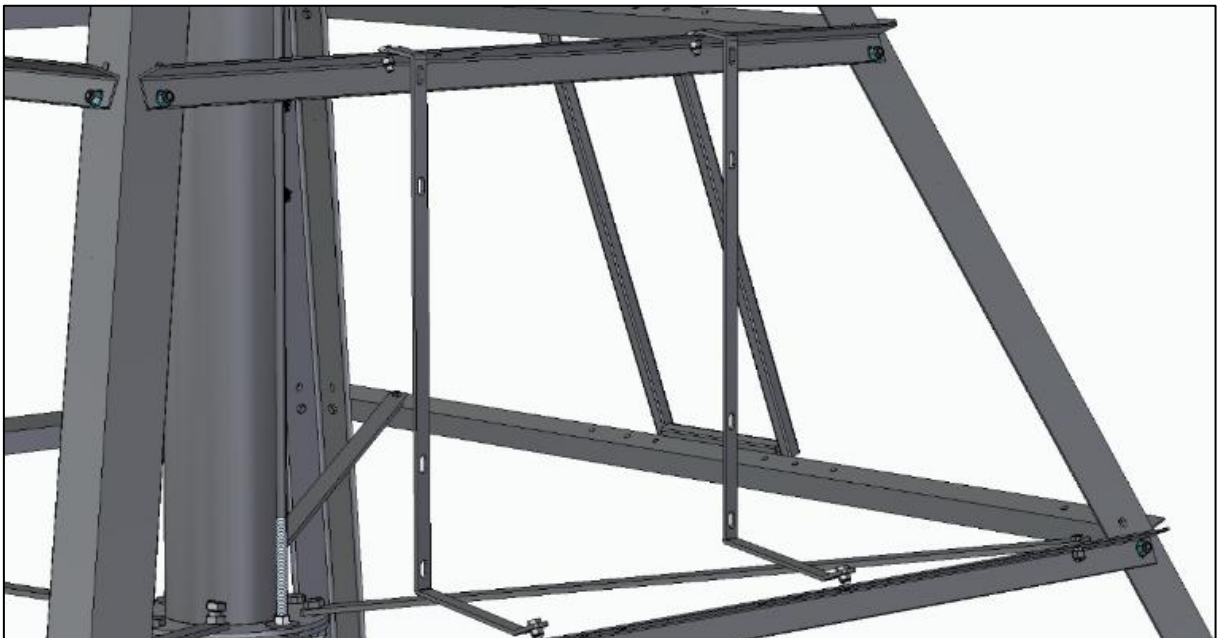
Figure 5 - Mounting of the cabinet brackets to the pivot's central tower.
