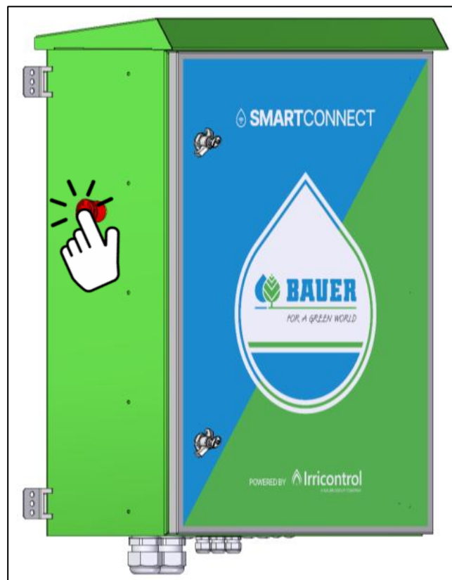
Figure 69 - Emergency Button Test.
