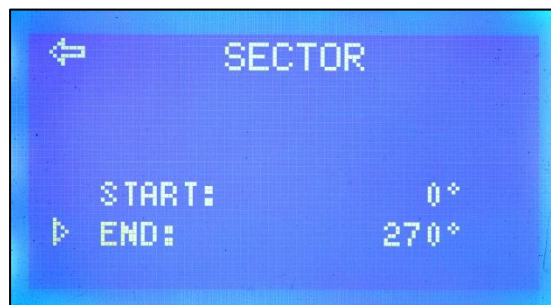
Figure 31 - Sector Parameter for pivots operating below 360°.
