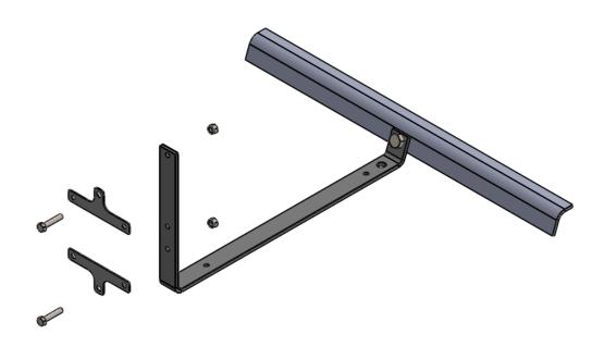
Picture 4: Fitting the smaller hanger to the inclined stand
