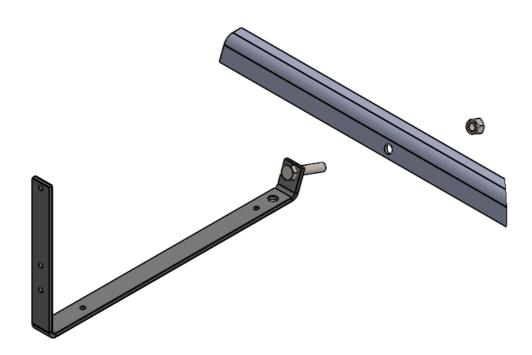
Picture 3: Fitting the inclined stand to the pivot
